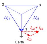
Figure 3.9: Vector diagram of the capacitive currents (also applies to harmonic currents)
