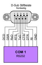
Figure 4.12: COM1 Serial interface
