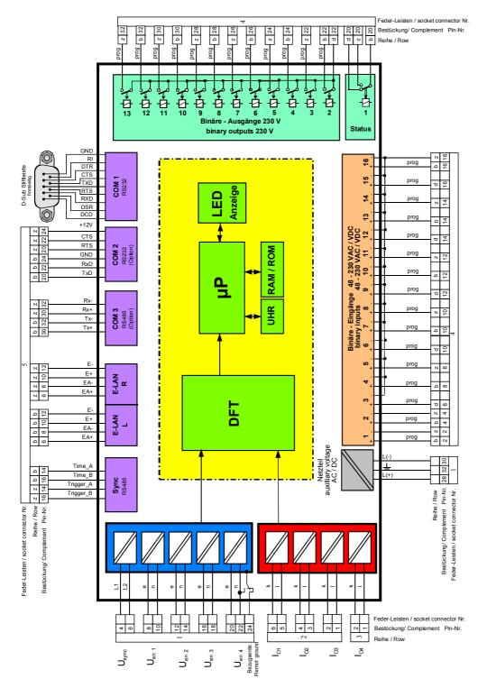
Figure 4.4: Contact assignment of the socket connectors
