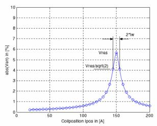
Figure 3.6: Resonance curve of the healthy network operation ("high-resistance asymmetry:  $Y_U = \omega \Delta C$ ")
