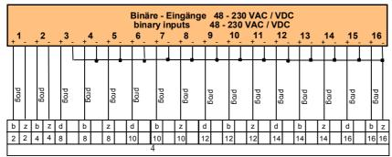
Figure 4.7: Socket connector 4: binary inputs
