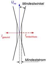
Figure 6.4: Minimum current and minimum angle
