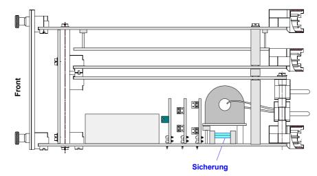
Figure 8.1: Changing the fuse on circuit board 1
