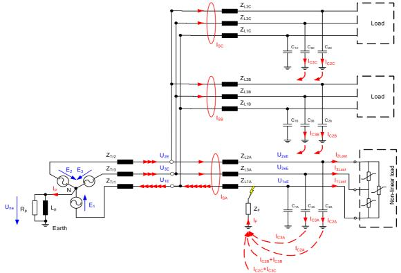
Figure 3.10: Network with three feeders and a single-pole earth fault in L1 of line A.
