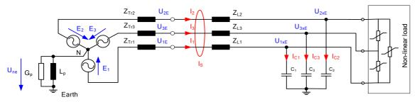
Figure 3.7: Simplified equivalent circuit diagram of the healthy network
