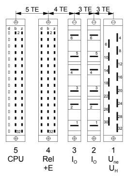
Figure 4.3: Location of the socket connectors (view from behind)
