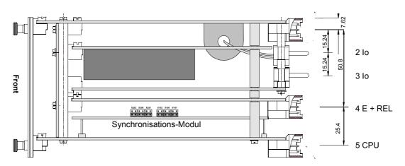
Figure 4.2: Location of the circuit boards and blade connectors (top view)
