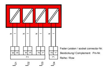
Figure 4.6: Socket connectors 2 + 3: current inputs
