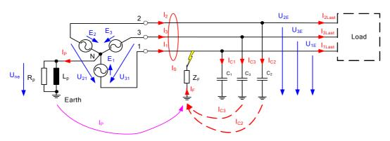
Figure 3.3: Simplified equivalent circuit diagram of the compensated medium-voltage network with single-pole earth fault
