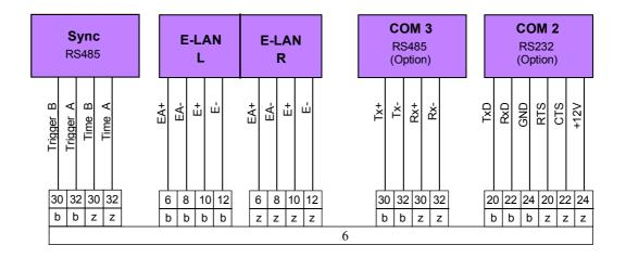
Figure 4.9: Socket connector 5: Communication COM 2, COM 3, E-LAN, time synchronisation
