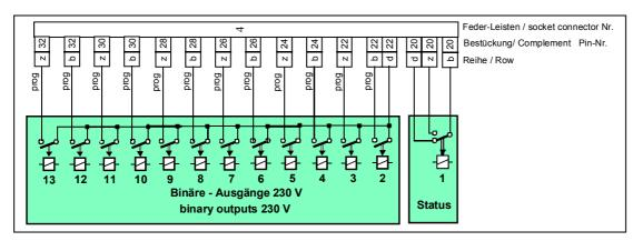
Figure 4.8:Socket connector 4: binary outputs BO
