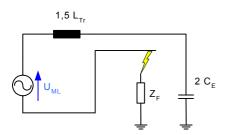
Figure 3.14: Equivalent circuit diagram for the charging procedure
