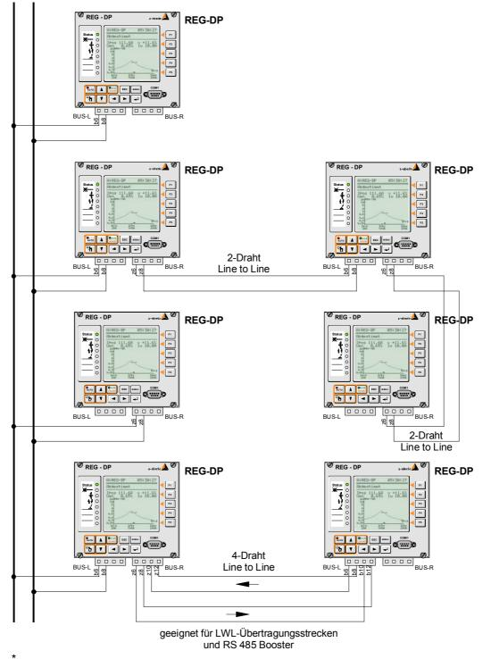
Figure 4.11: Possible E-LAN connection using REG-DP as an example
