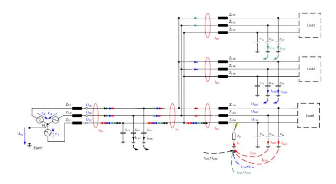
Figure 3.15: Network with feeder cable from the transformer to the busbar and three feeders
