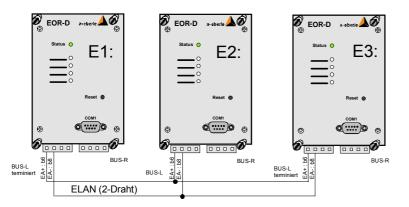
Figure 4.10: Example configuration for three EOR-Ds with ELAN two-wire connection
