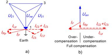
Figure 3.4: Vector diagrams for the single-pole earth fault according to Figure 3.3
