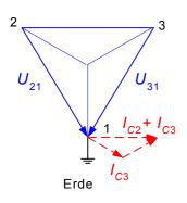
Figure 3.16: Vector diagram for the earth fault currents
