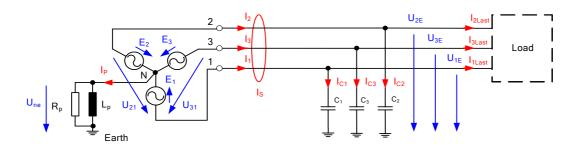
Figure 3.1: Simplified equivalent circuit diagram of the healthy compensated medium-voltage network
