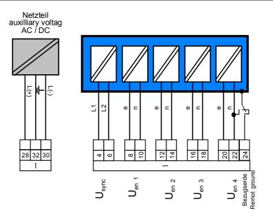
Figure 4.5: Socket Connector 1: Neutral earth voltage Uen1 ... Uen4, Usync and auxiliary voltage
